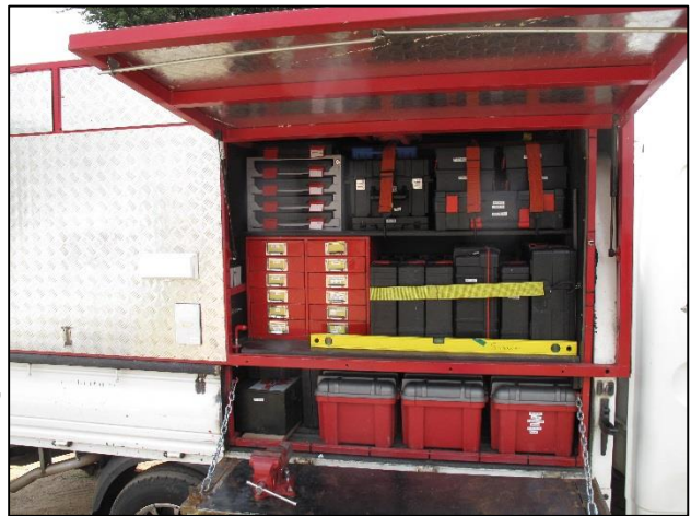
All hardware items and tools neatly stocked and catalogued. Note the vice fixed to the drop side.
