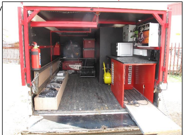
Hardware box (left) contains drawer runners, adjustable feet, etc. At the back is the cut-off saw, generator, extension leads & tools. Pull out rack for the fridge.
