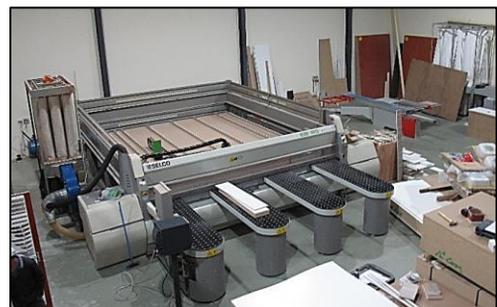
The beam saw and panel saw being commissioned
